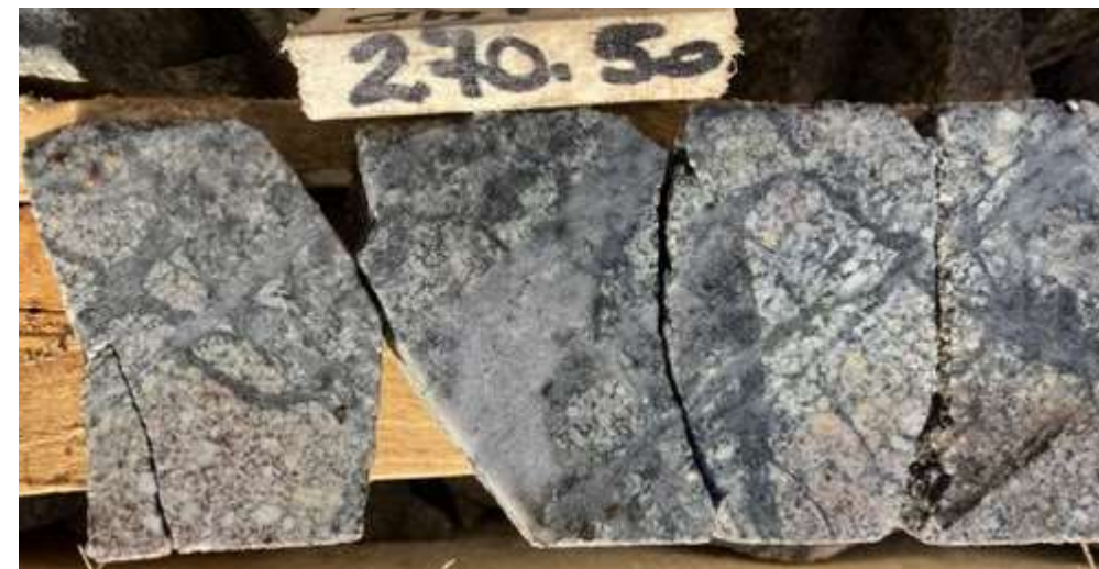
Hole PIU01: Multi-phase quartz veinlets in potassic altered inter-mineral diorite porphyry (270.5 m)
